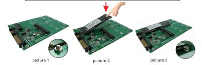
Step 1: Put copper nut on the same side of the NGFF connector; and fix M3x5mm screw from bottom to top of the adapter.
